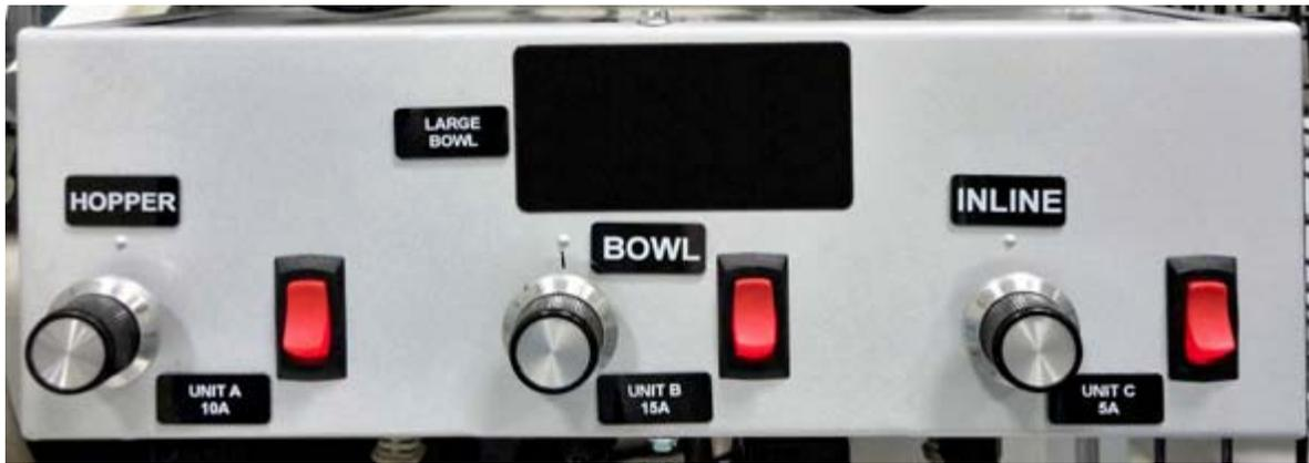
Photo 3. Per the 2012 edition of NFPA 79, Article 16.3, control devices, visual indicators, and displays used in the operator machine interface shall be clearly and durably marked with regard to their function either on or adjacent to the unit.
