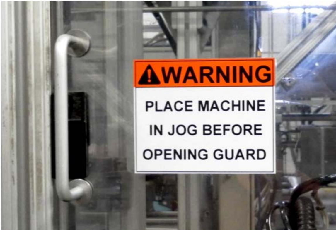
Photo 4. Per ANSI Z535.4-2011 6.3: A safety alert symbol, when used with the signal word, shall precede the signal word.
