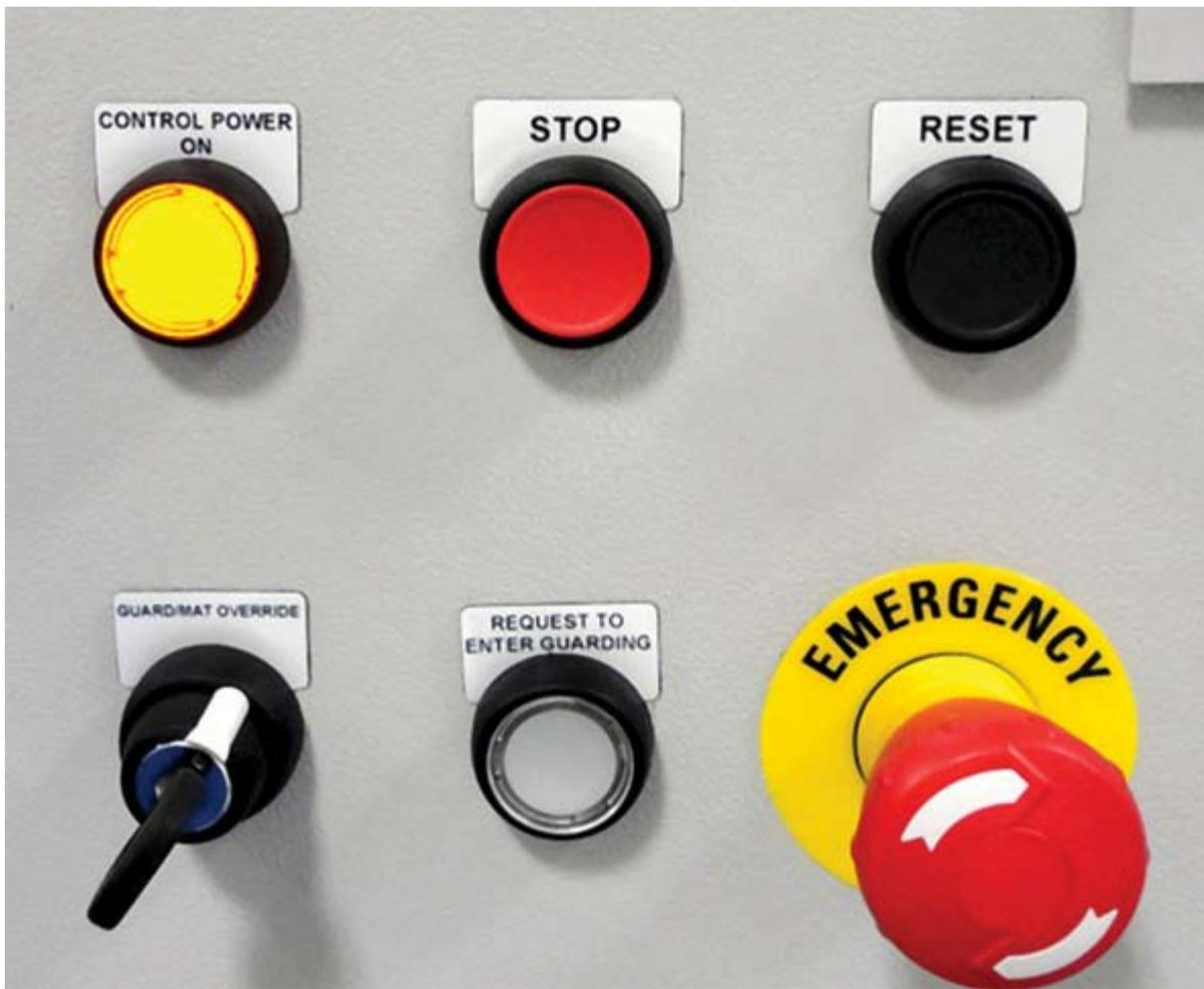
Photo 5. Even the emergency stop label is defined under NFPA 79-2011 Article 10.7.3 and is required to be yellow.
